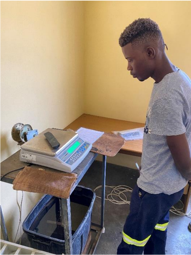
Figure 11-4 Apparatus for measuring density (SG) by the Archimedes principle
